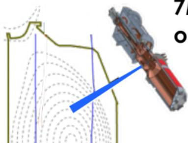
**7MW ECH ordered: directable electron heating or current drive, without fueling or torque**
