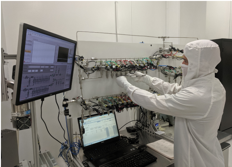
SULI student adjusts an automated mass spectrometer system as part of his research in the Inertial Fusion Technology division
